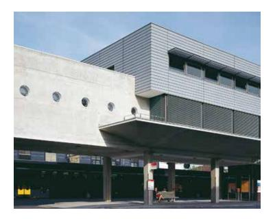
cladding, reminiscent of wooden façades. When exposed to light and shade, sharp contours appear because of its profile geometry. Contrary to the horizontal and vertical reveal panels, this system does not have any reveals.
