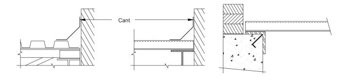
**Detail 9: Roof Deck at Insulated Sheet Steel Wall**
