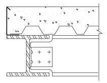
**Detail 6: Framing Around Interior Columns**
