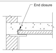
**Detail 5: Pour Stop Angles at Perpendicular and Parallel Conditions**
