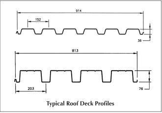
removable formwork. There were some situations, however, where the deck did not have a concrete cover and was the sole load carrying element. The name for this type of deck is floor deck, or non-composite deck. In the 1960's, floor deck products were developed that
