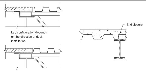
Detail 3: Side Condition - Beam at Lower Level Than Girder
