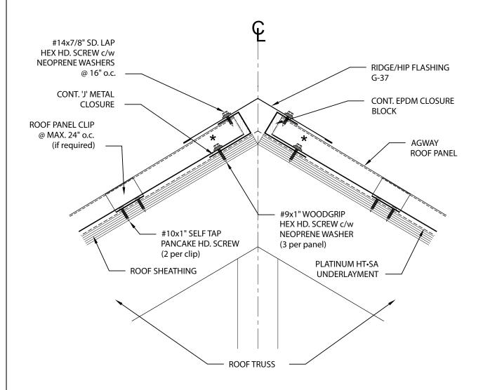
\* NOTE: ROOF PANELS MUST BE ALLOWED TO EXPAND AND CONTRACT, THEREFORE FASTEN PANELS AT ONE END ONLY.
