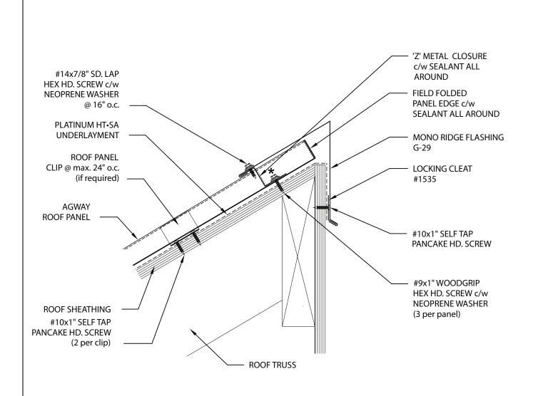
\* NOTE: ROOF PANELS MUST BE ALLOWED TO EXPAND AND CONTRACT, THEREFORE FASTEN PANELS AT ONE END ONLY.
