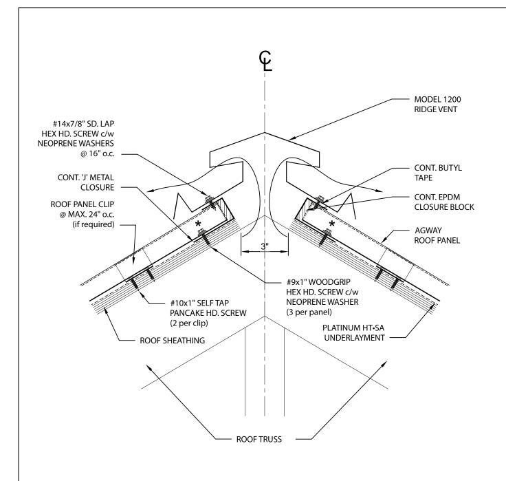
\* NOTE: ROOF PANELS MUST BE ALLOWED TO EXPAND AND CONTRACT, THEREFORE FASTEN PANELS AT ONE END ONLY.
